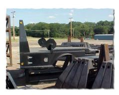
If you use your truck for a truck, then you'll appreciate all the standard features on a Bradford Built truck bed; things like 1/8" thick tread plate floor, a 30,000 lb rated gooseneck hitch and the incredibly strong receiver type bumper hitch. Chain "keyholes" in the headache rack make it easy to secure any load. The sealed beam lights are flush mounted and there is a 7-pole plug-in for your trailer.
